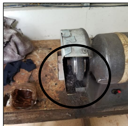
Figure 19: Unshielded Grinding Wheel
