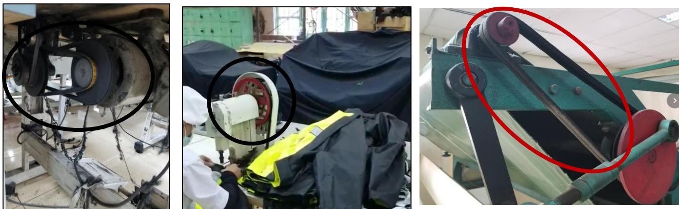
Figures 20-22: Lack of Guarding on Belt-Driven Machines
