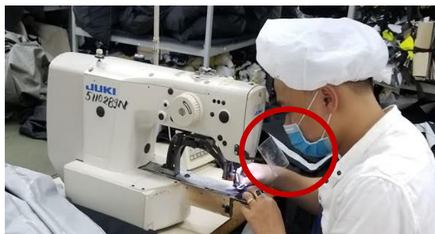
Figure 23: Sewing Machine with Guarding
