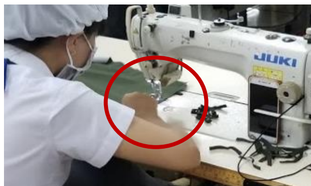
Figure 24: Lack of Guarding on Sewing Machines
