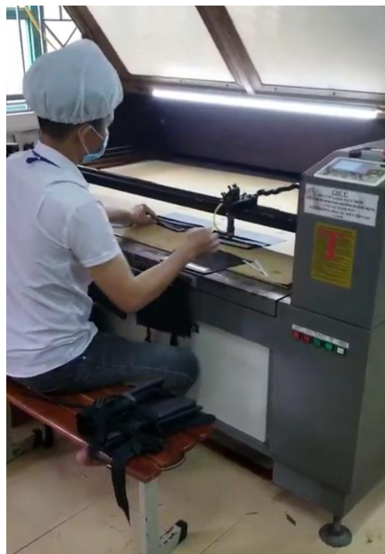
Figure 34: Laser Cutter Operated by Worker with Lid in Raised Position
