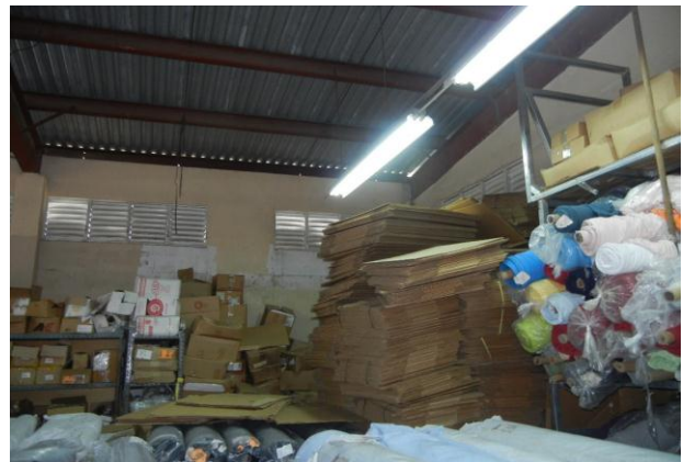
Left: Pattern cutting saw with no grounding that produces sparks when filing edge. Right: Large accumulation of stacked combustible cardboard and fabric.
