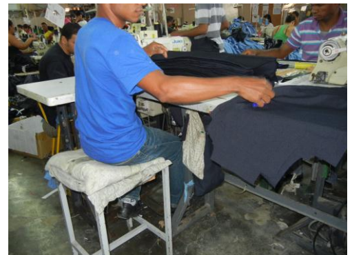
Bottom left: Chair with unsafe makeshift height adjustment by sewing operator.
