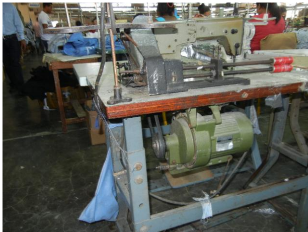
Top left: Tensioner hot surface with makeshift adhesive tape guard to protect against burns. Top right: Unguarded belt with exposed nip point on maintenance room machinery, Bottom left: Unguarded belt drive on sewing machine. Bottom right: Unguarded belt pulley on air compressor.
