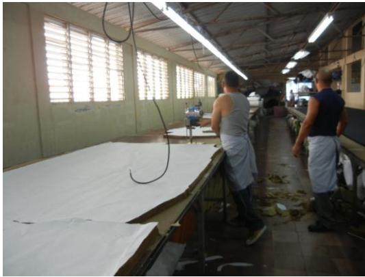
Left: Energized electrical cord accidentally pulled off pattern saw.
