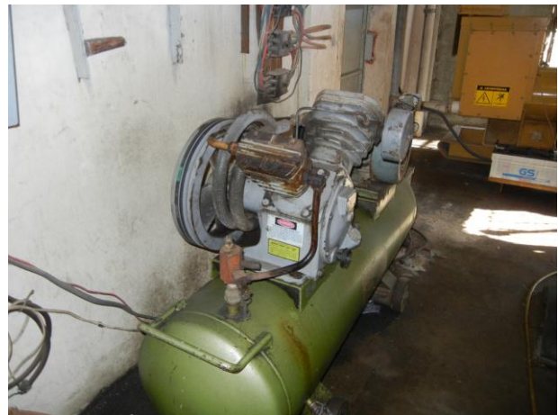
Top left: Tensioner hot surface with makeshift adhesive tape guard to protect against burns. Top right: Unguarded belt with exposed nip point on maintenance room machinery, Bottom left: Unguarded belt drive on sewing machine. Bottom right: Unguarded belt pulley on air compressor.
