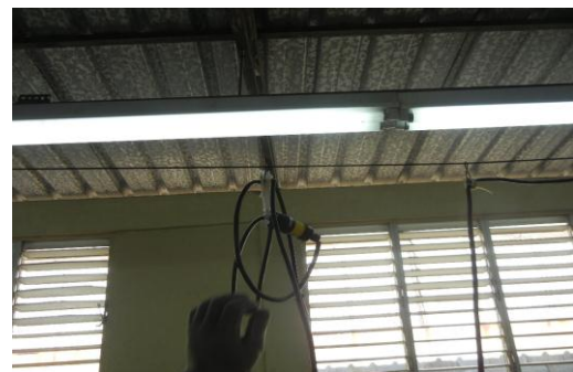
Jam on cord zip line that caused cord to break off.
