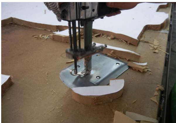
Left: Pattern cutting saw with no grounding that produces sparks when filing edge. Right: Large accumulation of stacked combustible cardboard and fabric.
