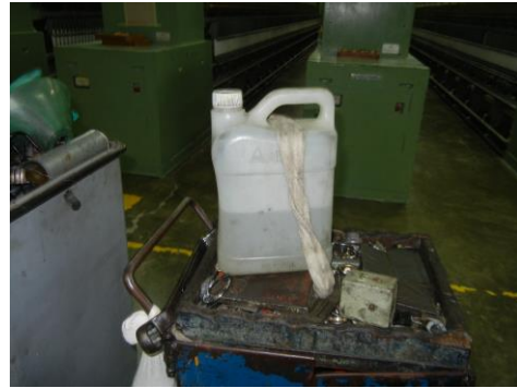
Unlabeled thinner container on maintenance cart.
