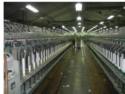
Unguarded "continuas" spinning machines with worker.
