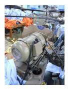
• Also in Building One, the drop cord of one sewing machine is pulled, conductors are exposed, and insulation is cracked.
